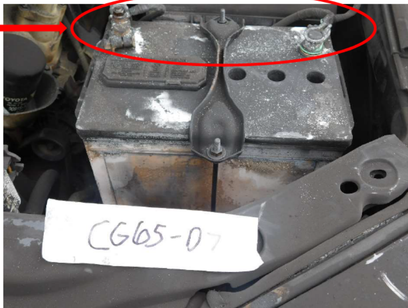
Figure 10. A connected battery on a vehicle from deck 7 of the HOEGH XIAMEN taken on July 12, 2020, provided by the Coast Guard. The vehicle was originally towed onto the vessel by stevedores.
