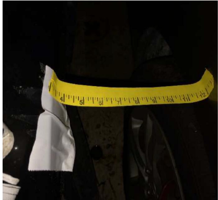
Figure 6. Spacing between vehicles on deck 5 of the HOEGH XIAMEN taken on June 11, 2020, provided by the Coast Guard.
